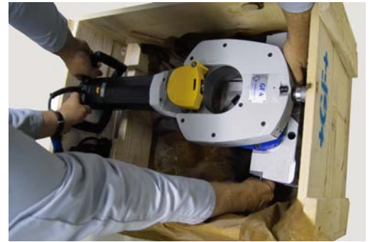
Transport and fit the machine with the aid of a second person or a crane or similar device.
