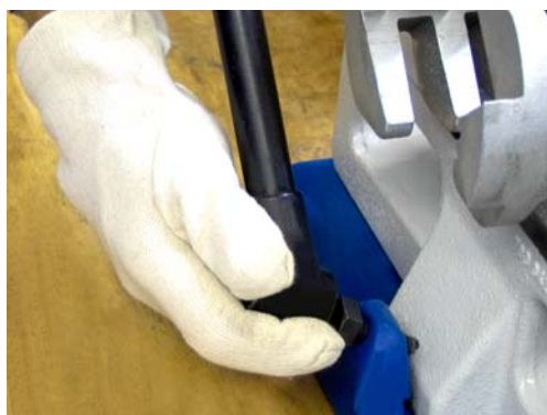
Tightening the GF 4 quick mounting plate
